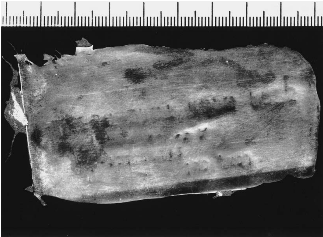
FIG. 4—Polymer cast taken of the internal side of the clear plastic window of the plastic credit card holder.
